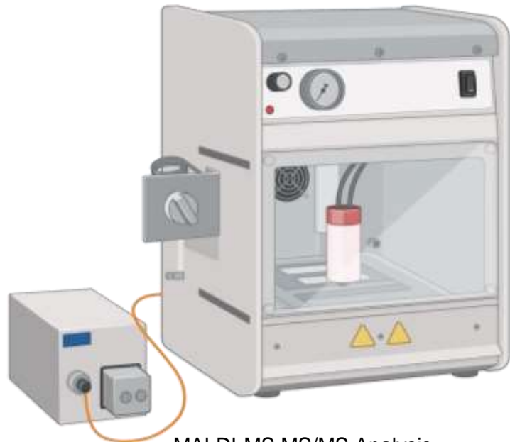
MALDI-MS MS/MS Analysis Matrix-assisted laser desorption/ionization Tandem Mass spectrometry
